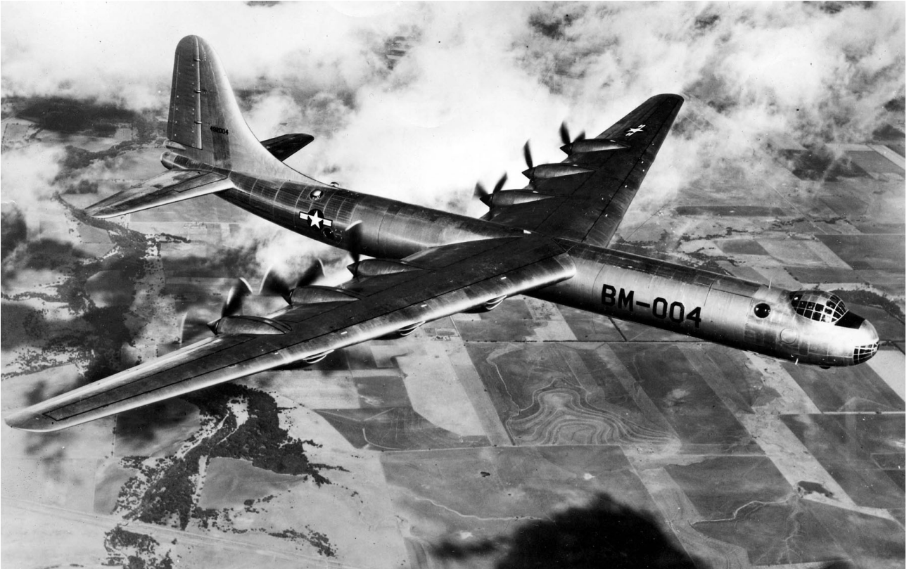
Convair B-36A-1-CF (S/N 44-92004, the first -A model built) in flight. (U.S. Air Force photo)
