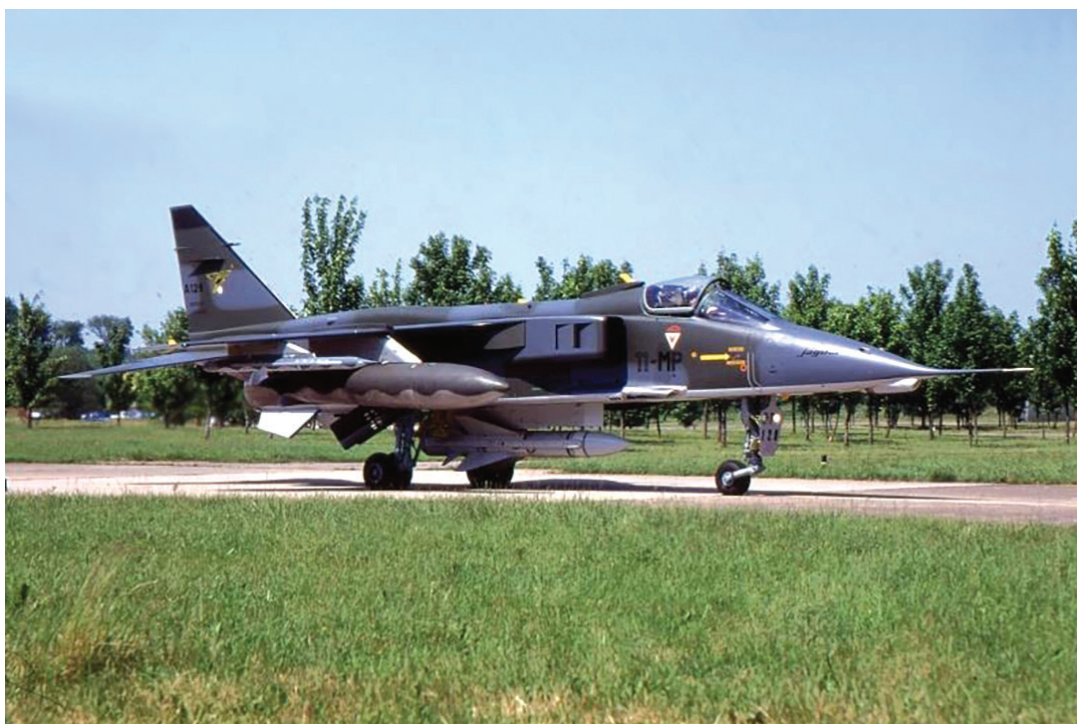
Le Jaguar A 129 en configuration missile anti-radar, emportant un missile AS 37. Crédits P. Bigel.
